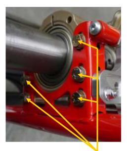
Bearing carrier fixing bolts
