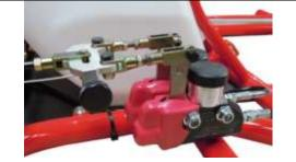
Front and Rear Combination Foot brake Master Cylinder (Open system)
