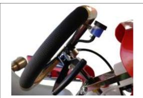
Front Hand brake Master Cylinder (Open system)
