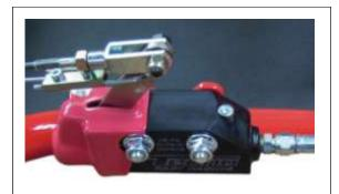
Rear Foot brake Master Cylinder (Closed system)
