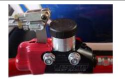
Rear Foot brake Master Cylinder (Open system)
