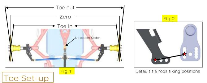
Before fixing the rod ends to the stub axles and the steering column, make sure that the thread of the rod ends are completely screwed by hand to each side of the tie rods. One side of the tie rods have reverse thread so turn it counter-clockwise to tighten. The length of the two tie-rods are same or slightly different depend on the frame. If different,
