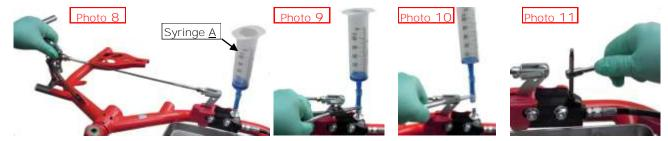
14. Operate the lever of the master cylinder. The lever must be stiff and not have the play. If no, repeat step 1 to 12.
